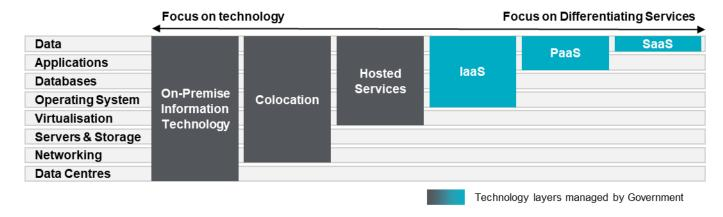
Figure 2 - Cloud enables a focus on differentiating services
